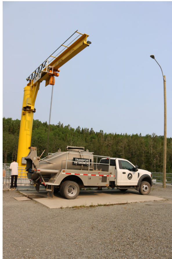
47 The crane places the cage on top of the transport truck where the fish is dispensed into the steel drum.
