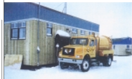
Wastewater being removed by a tanker truck equipped with pumps
